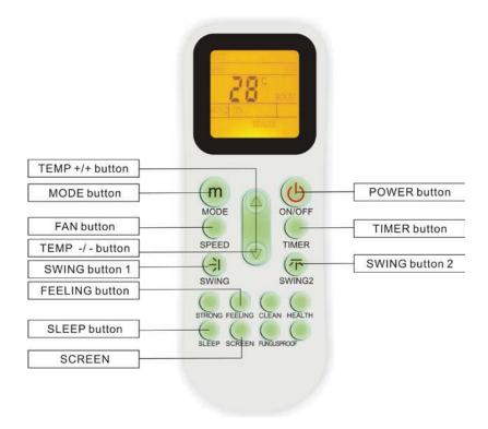
POWER button: Switch the unit ON/OFF.
