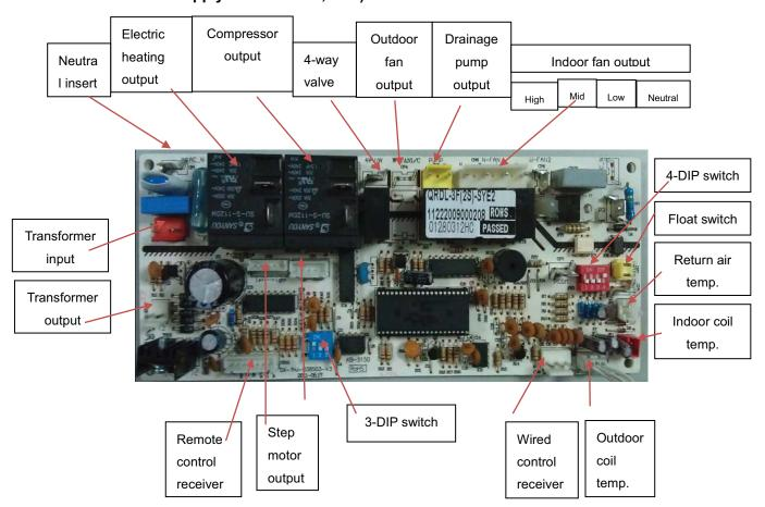
Introduction of control board QRD-SN3F(2S)-SYE1 sockets (Indoor unit) (match with the outdoor unit which the Power supply is 380V-415V, 3PH)
